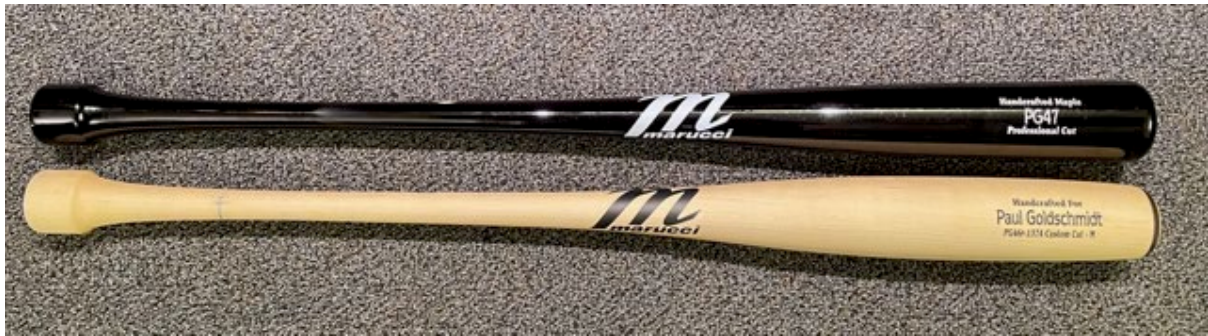
Figure 1: Two of the bats used in the present study: a standard bat (top) and torpedo bat (bottom).
