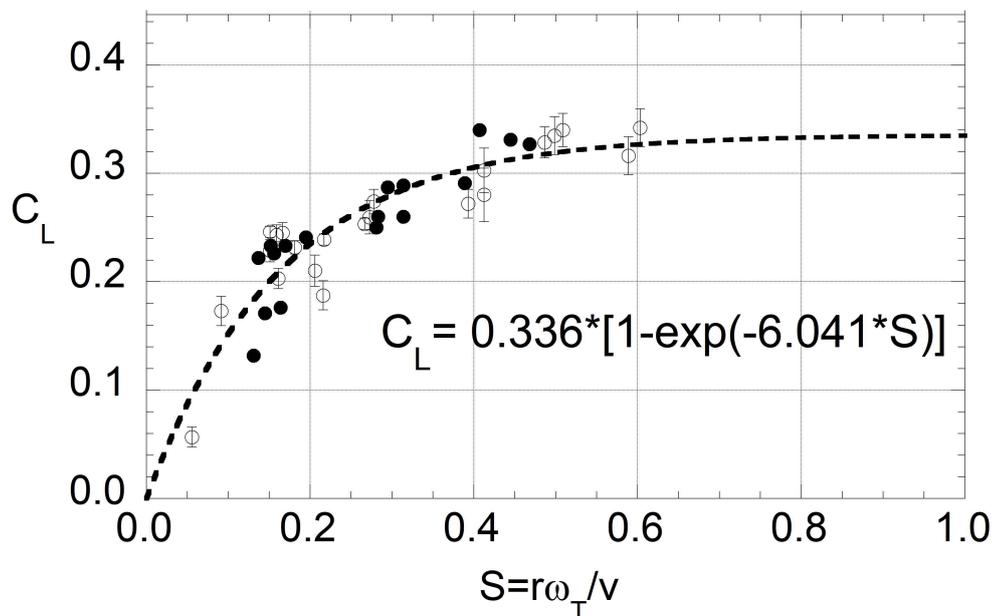
FIG. 1: Experimental values of  $C_L$  as a function of  $S$  for the special case purely transverse spin,  $\sin \theta=1$ . The data come from motion capture experiments taken at speeds in the range 80-100 mph, including data from Always<sup>1,2</sup> (closed points) and Nathan (open points).<sup>3</sup> The data were parametrized by the function  $C_L = f(S) = A(1 - e^{-BS})$ , with  $A$  and  $B$  determined from a non-linear least-squares fit (black curve), with  $A=0.336$  and  $B=6.041$ .
