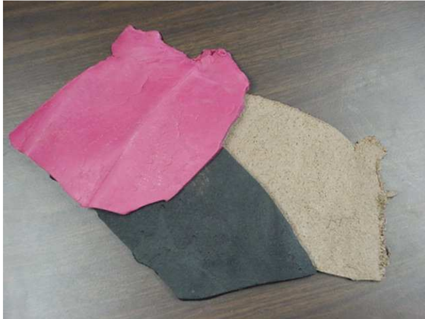
Figure 4. Samples of the #6, black-rubber and compressed-cork sheets
