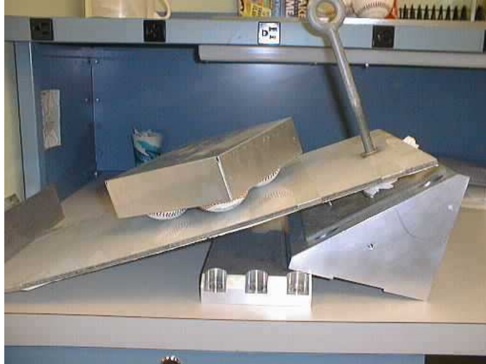
Figure 3. 4-Ball Friction Test Set-up
