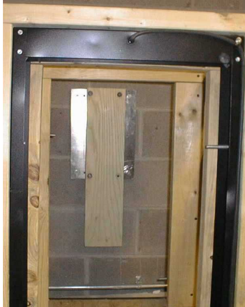
Figure 2. COR Wall Test, Target and Speed Gate
