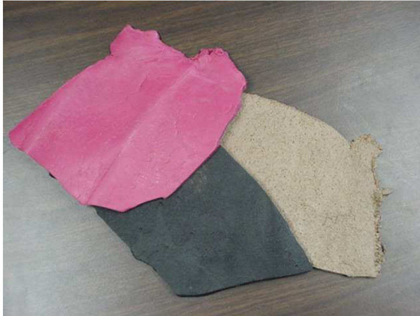
Figure 4. Samples of the #6, black-rubber and compressed-cork sheets
