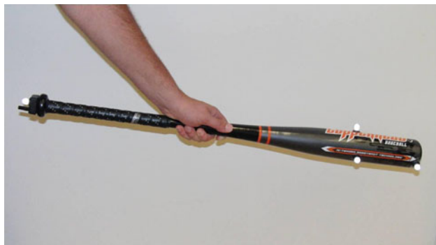
Fig. 12 Instrumented bat used for benchmarking study. Five reflective markers (four of which are visible in this image) were used with VICON motion analysis system to determine the velocity of the sweet spot. The knob-mounted IMU was used simultaneously to determine the velocity of the sweet spot
