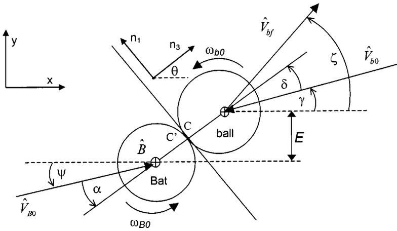
Fig. 1. Two-dimensional impact schematic. The bat-ball contact occurs with the bat horizontal, but with both vertical and horizontal components of bat and ball velocities and bat and ball spin. The batted ball speed  $\hat{V}_{bf}$ , launch angle  $\zeta$ , and spin  $\omega_{bf}$  are functions of pre-impact bat and ball speed and spin, the angle  $\gamma$ , and the two primary batter controlled parameters,  $E$  and  $\psi$ .
